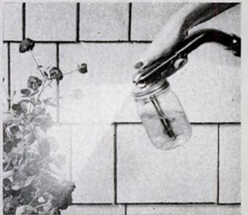
Sprayer is used for insecticides, moth-proofing fluids, painting and liquid wax. Adjustment screw regulates intensity.
