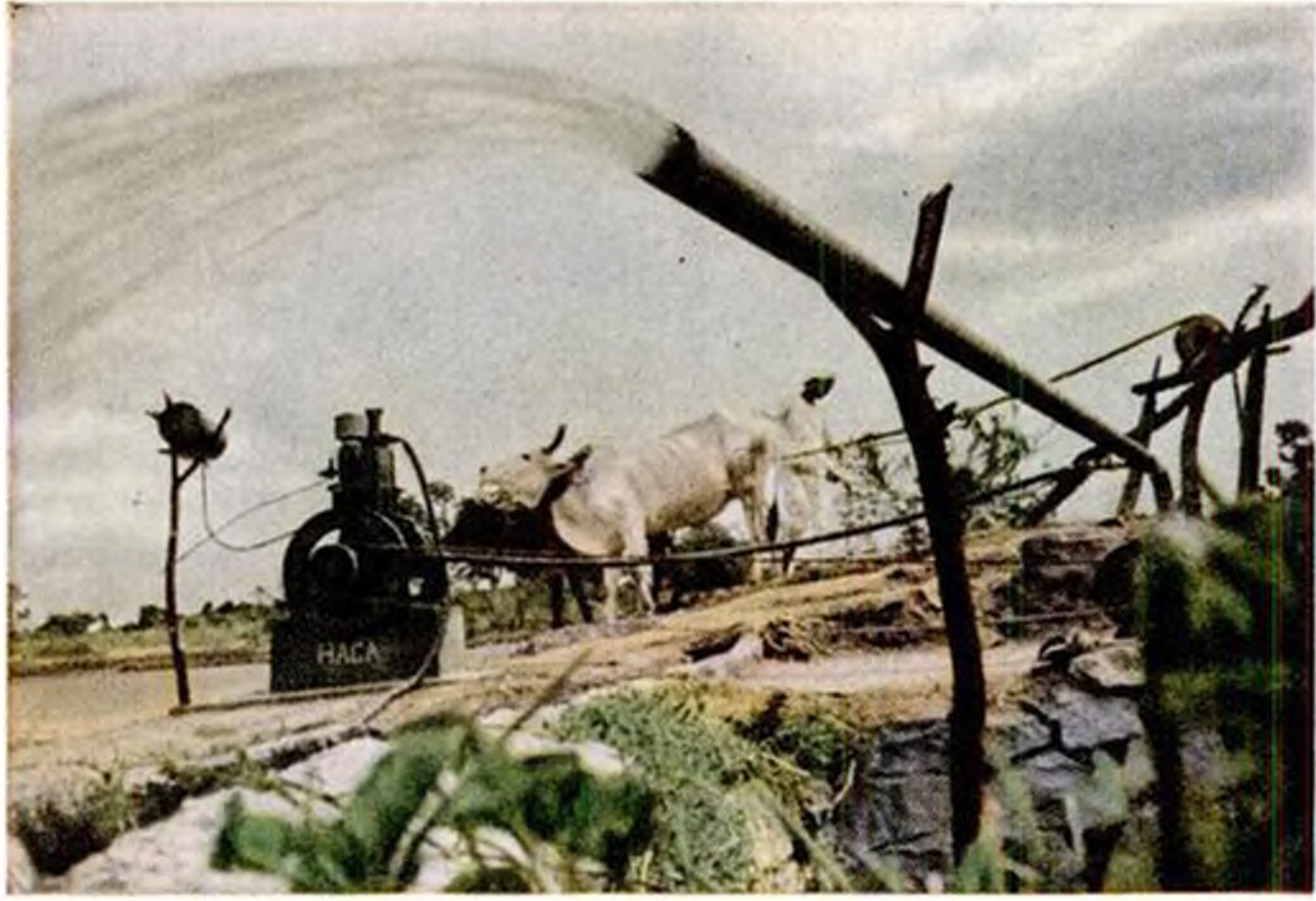
IN POWER TEST farmer pits engine-driven pump, bought with $630 state loan, against traditional bullocks and buckets to see which draws most water.
